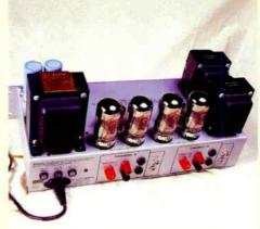
Unlike transistor amps, valve versions need 4ohm/8ohm taps on their output transformers to match loudspeakers of different impedances.
