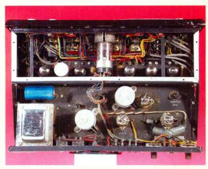
The Empress 556 self-powered pre-amp is a world away from the simplicity of some valve gear. Its plethora of switches and potentiometers can cause lots of noise unless they're properly cleamed.
