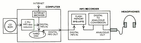
At present MP3 recorders load data-reduced MP3 songs into memory from a computer. Song and track details are shown on a display. Music is played out of memory through a DAC and amplifier to headphones or an earpiece.
